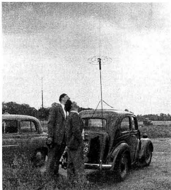
This capacity hat on G3JIP/M's aerial aroused considerable interest at the Harlow Mobile Rally on September 1.
